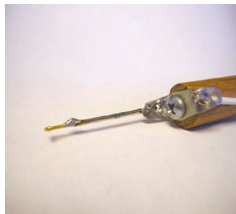
Figure 1b. Axial pogo pin at opposite end
