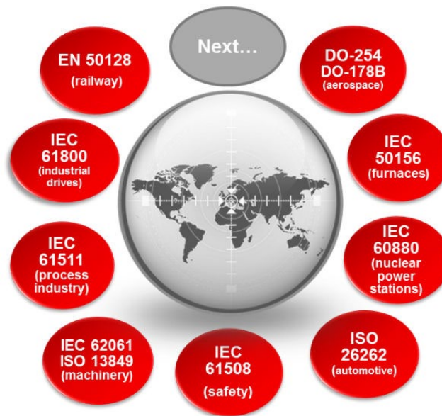
Figure 2 End-equipment-specific functional safety standards
