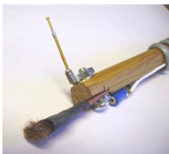
Figure 1a. Broom and radial pogo pin
